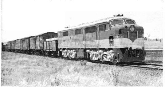
NEW South Australian diesel-electric locomotive 945 passes through Victoria on its way from Sydney—at the head of a goods train to Adelaide. Its bogies had been changed at Bandiana from 4' 8½" to 5' 3" gauge.
