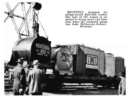
the Department is constructing ten 45 ft. long bogie flat top container wagons and some of these are already in service. This bogie vehicle has a total load capacity of 44 tons and can carry—
