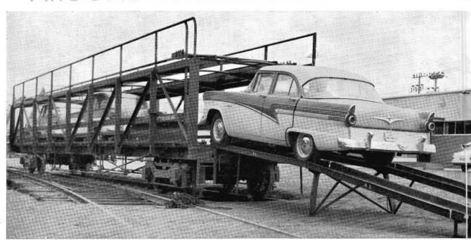
UNDER test at Ford Motor Company's Works, Geelong, was this new V.R. two-tier motor-car carrying rail wagon. Portable ramps were us demonstration purposes; fully or semi-fixed ramps will be provided at loading and unloading points. Successful initial trip was on a recent bourne-Adelaide goods train.
